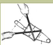
Figure BV4b. Using setting tool
